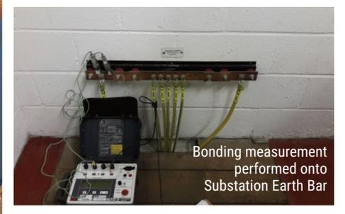
Bonding measurement performed onto Substation Earth Bar
